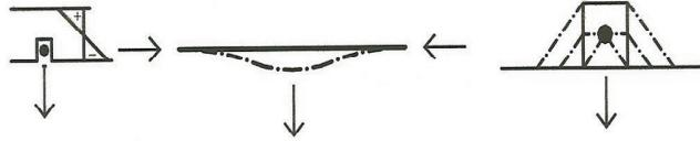
**Fig. 8:** Failure by rupturing of reinforcement from masonry chases
