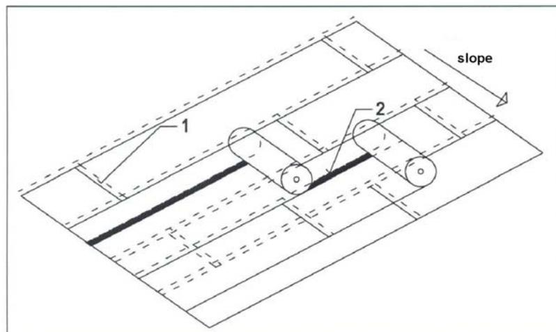
Fig. 3: Types of overlaps (1 - frontal, transversal, 2 – side, longitudinal)
