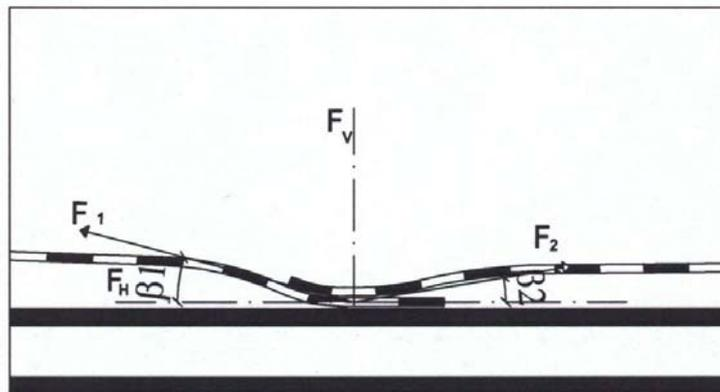
Fig. 2: Linear shear forces occurring in overlaps of bitumen sheets
