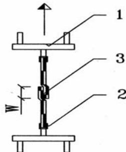
Fig. 4: Overlap shear resistance test, 1- testing instrument's frame, 2 – instrument's jaws, 3 – test specimen
