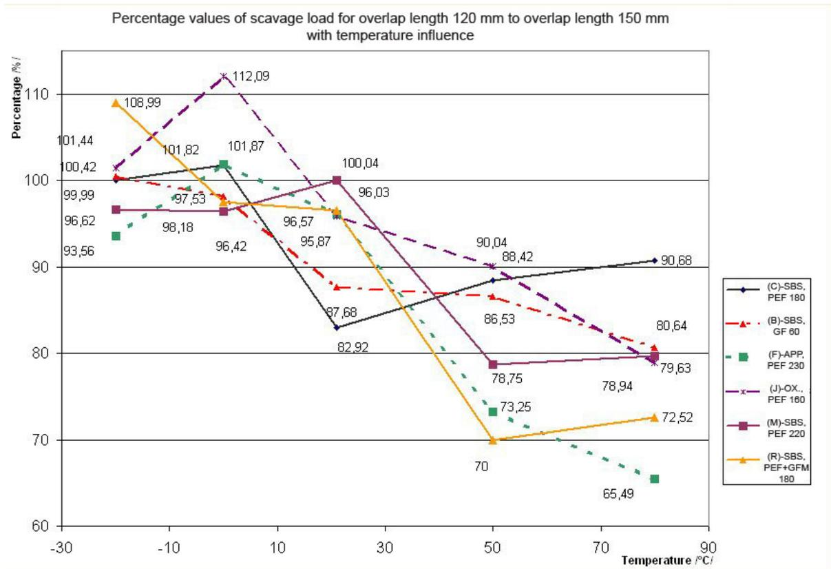
Fig. 6: Influence of temperature to dependency of ratio between overlap dimension for 120 and 150 mm
