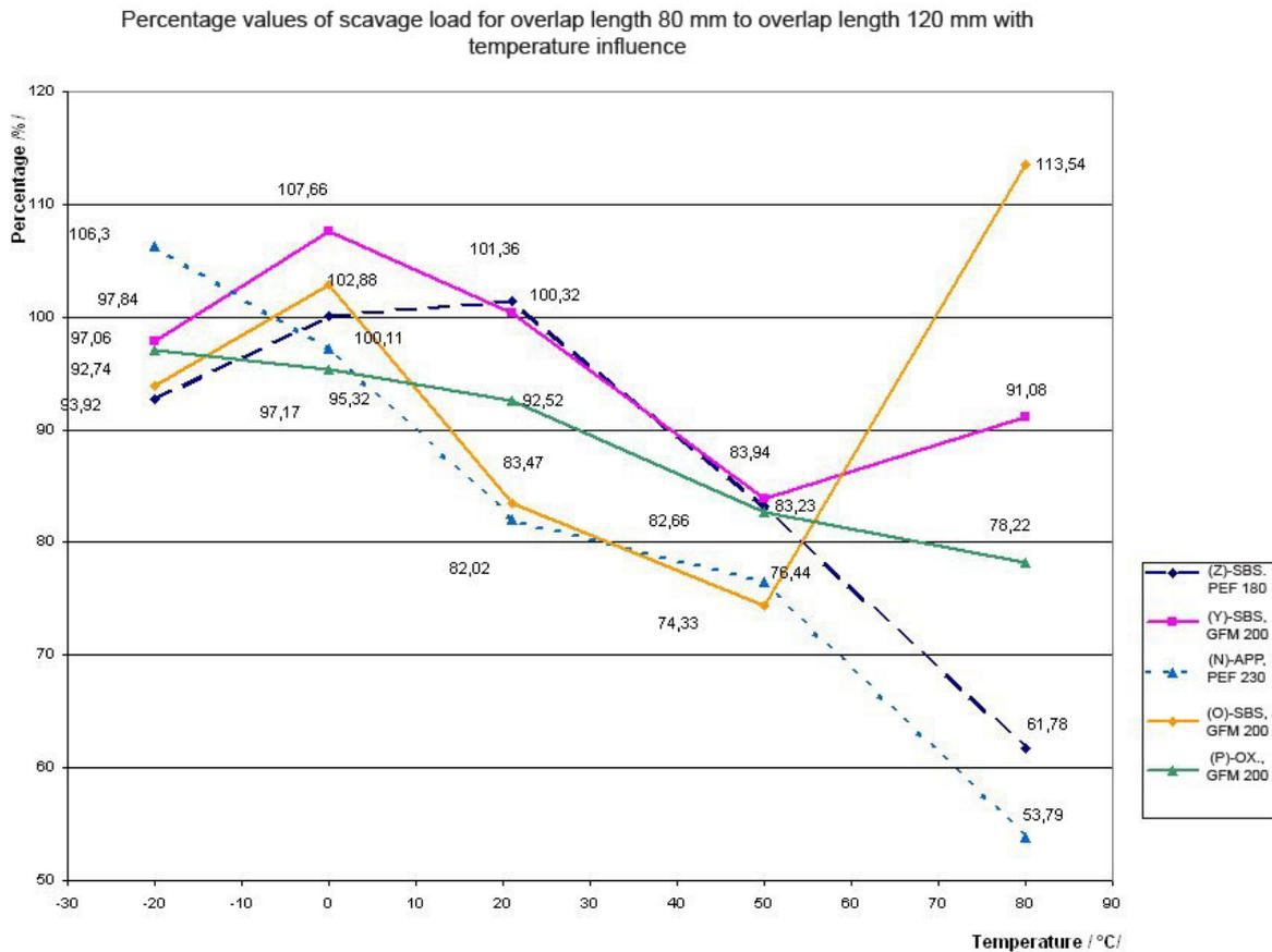
Fig. 5 - Influence of temperature to dependency of ratio between overlap dimension for 80 and 100 mm
