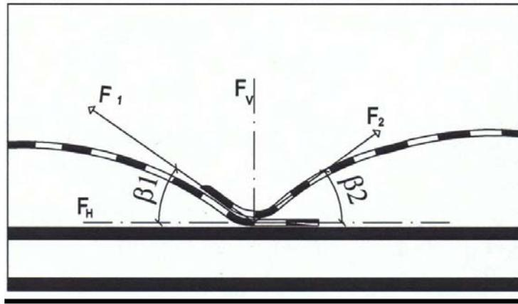
Fig. 1: Tangential forces occurring in overlaps of bitumen sheets
