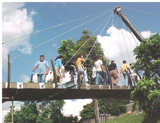
Figure 2: Loading test with “organized” pedestrians
