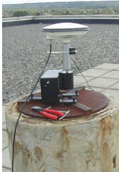
Figure 8: Illustration of the EMO with GPS rover antenna and accelerometer
