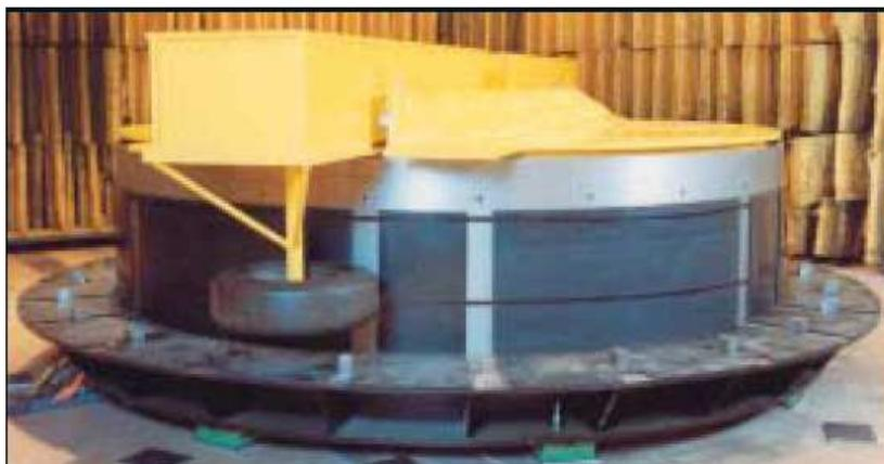
**Figura 8:** Tyre/Pavement Test Aparatus (TPTA)
